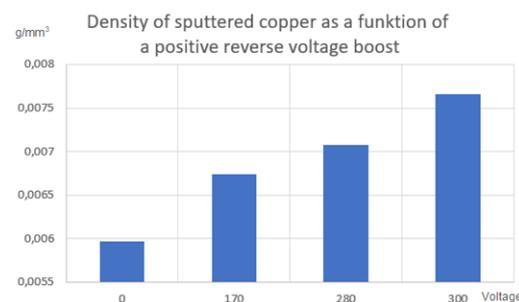
Both plasma power supply developments with this positive reverse pulse voltage, the **PLASMA TEC Ap** and the **HiPIMS hiP-V** have been initiated by- and are available through **4A-PLASMA®**, an engineering consultancy for Plasma Power Technology.
